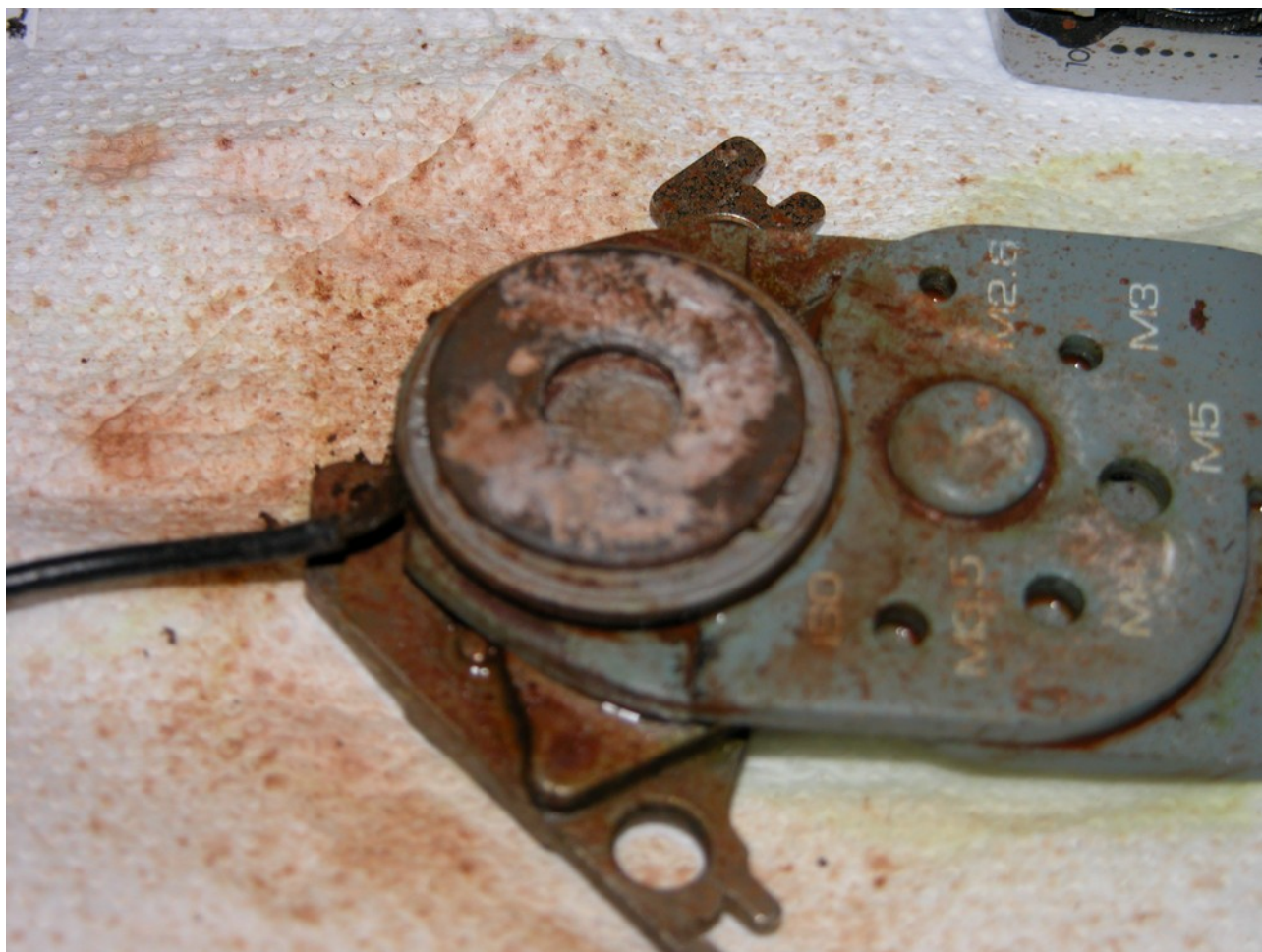
Figure 3.2.1: White sodium carbonates on the top cathode. Photo inadvertently blurred.
