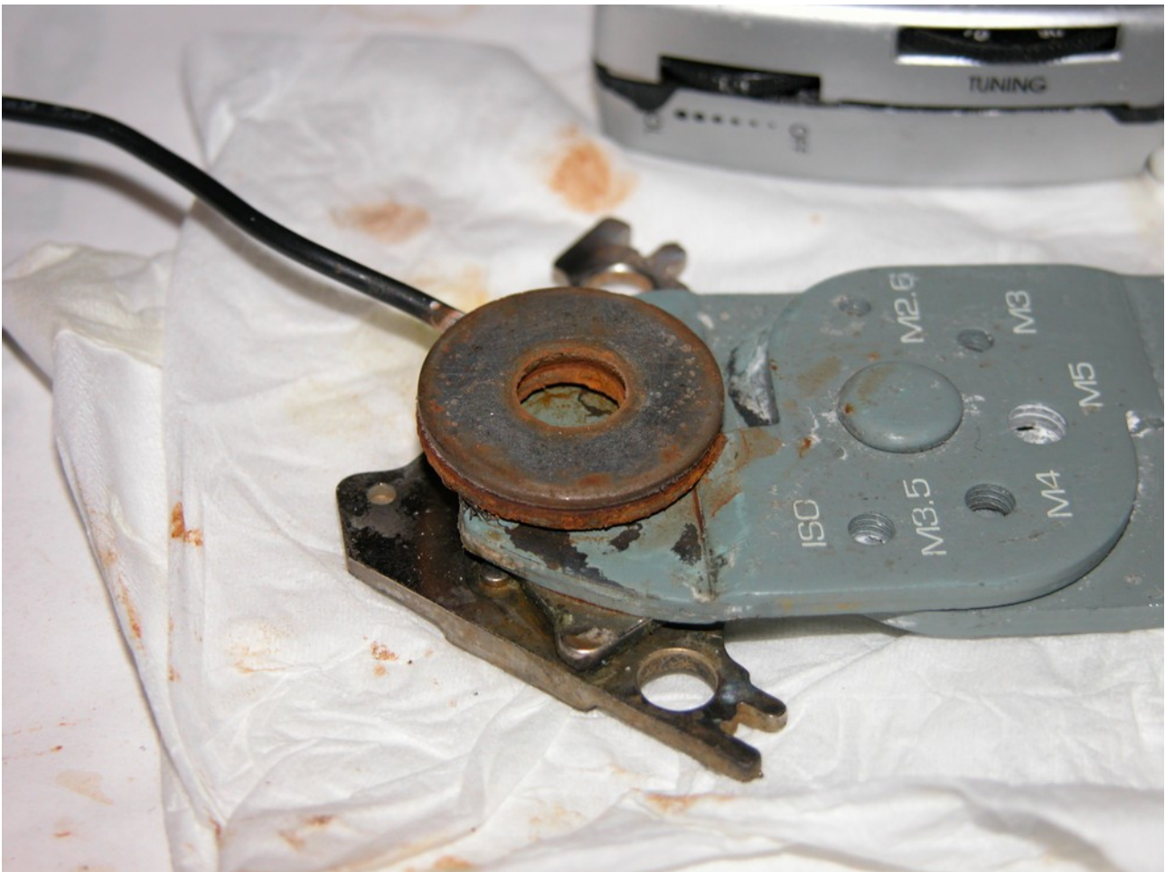
Figure 1.1.1: Ferritic steel washers as electrodes; top cathode, bottom anode. No electrolyte used.
