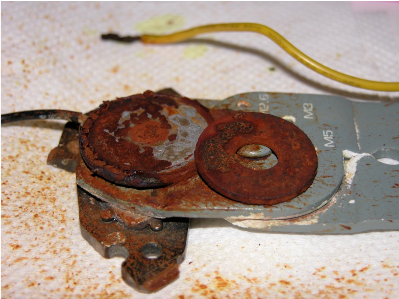
Figure 4.4.2: Electrodes disassembled. Some larger hematite pieces got stuck to the cathode presumably when I separated it from the anode.
