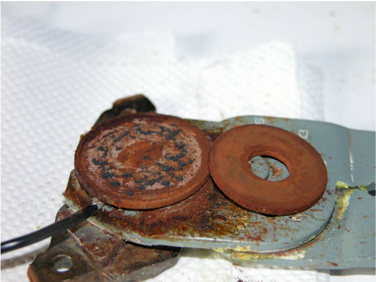
Figure 6.1.2: Graphite powder added, before being crushed and redistributed between both electrodes.
