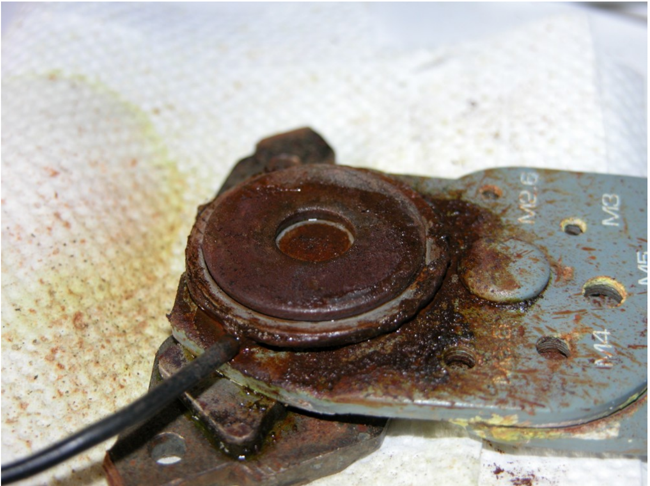
Figure 6.1.3: Hematite from the electrodes slowly disappearing.
