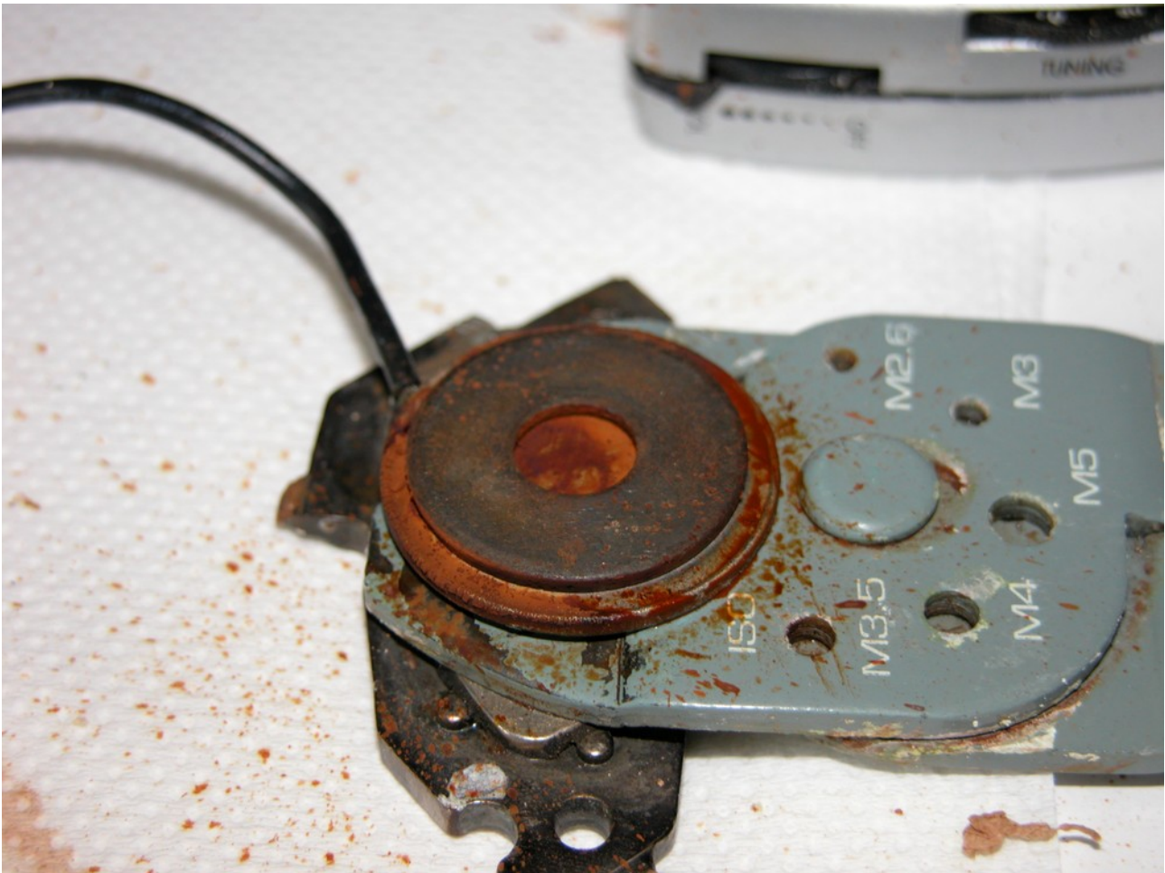
Figure 4.1.4: Exposed surface of cathode manually cleaned to achieve better conduction with the corresponding wire and avoid shorts.
