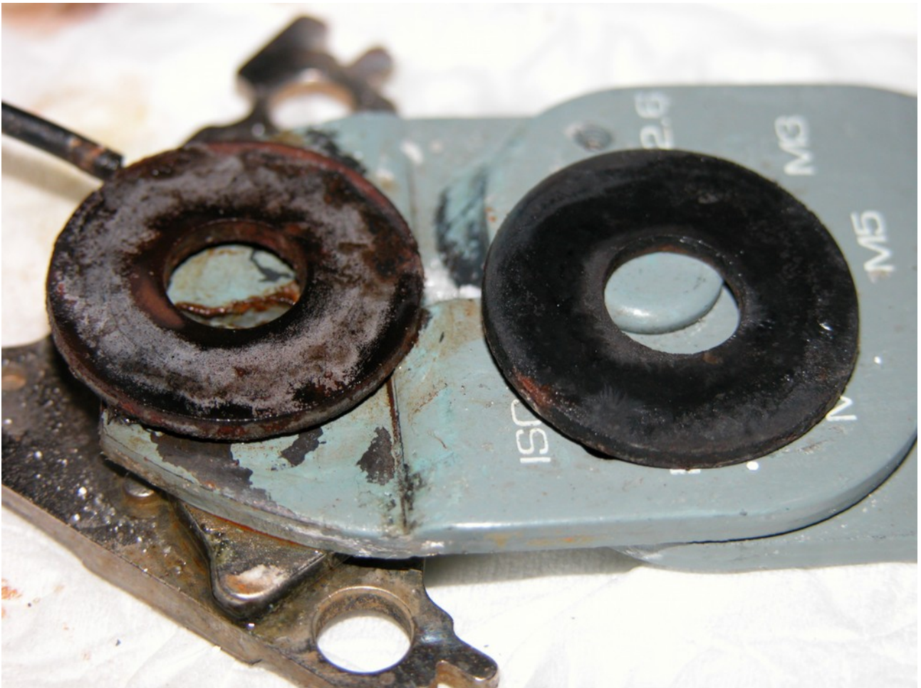
Figure 1.2.2: Electrodes after a longer period of operation using an electrolyte solution instead of just tap water.
