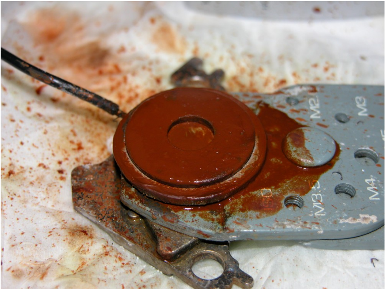
Figure 1.2.5: New arrangement with flipped coin after a while of operation. Rust production was intense and bubbling caused the top part to also become partially covered with it. Electrolyte was only minimally initially added.
