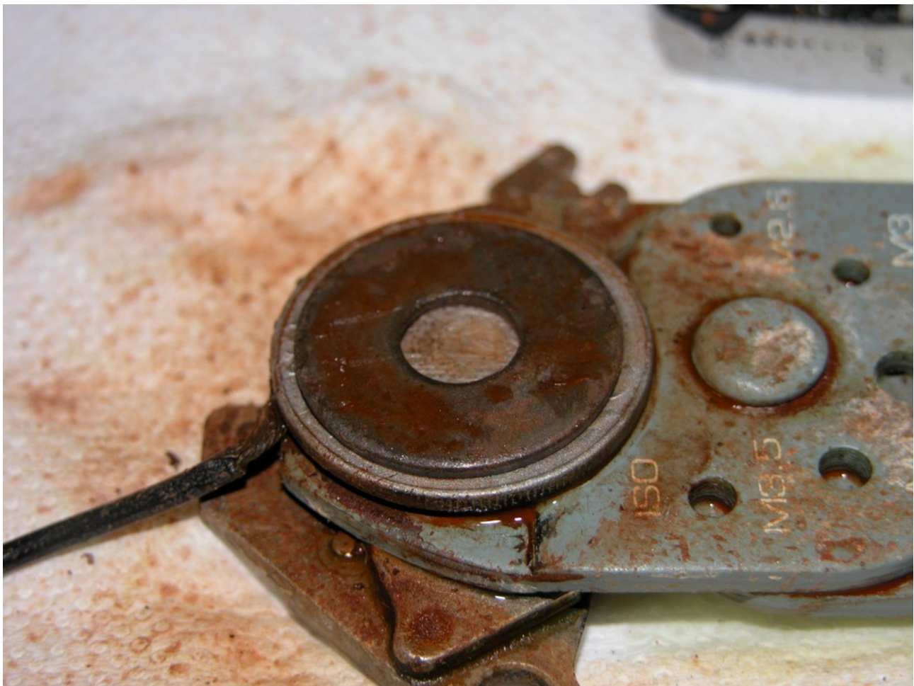
Figure 3.1.7: Electrode assembly after the experiment was terminated. Except for splatters around the testing area (which might be a problem with hydroxides) the electrodes themselves seem relatively clean compared to the first experiments in this series where I only used tap water.
