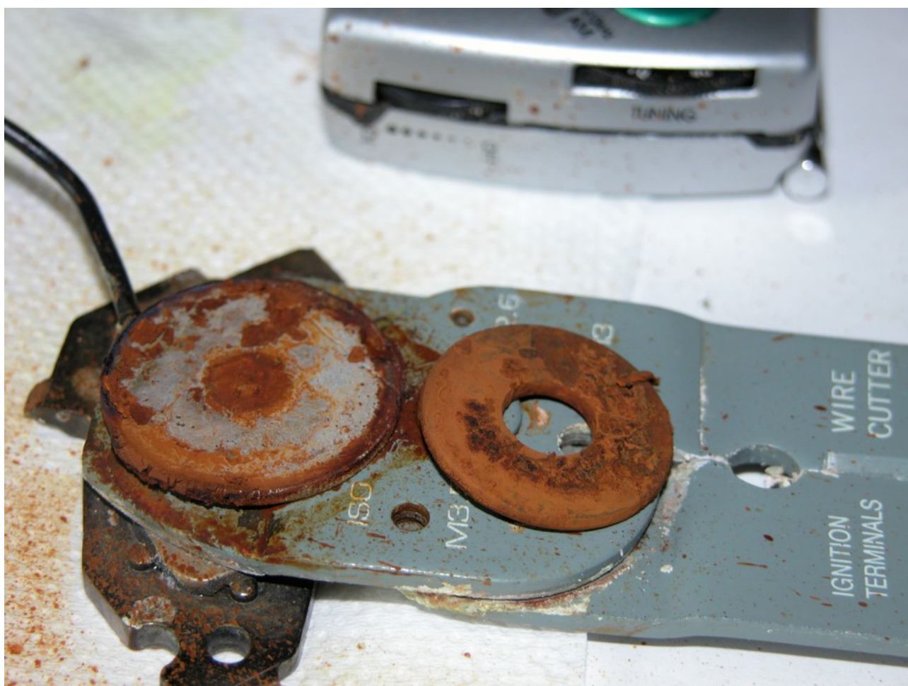
Figure 4.2.2: Upon inspection, the electrode interface also appears to be composed of dried material, mainly hematite. I have not separated the electrodes during the experiment.
