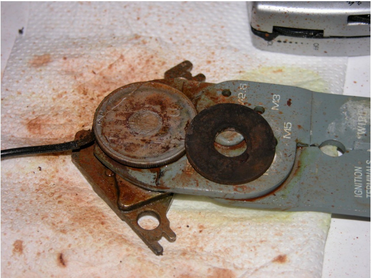
Figure 3.2.2: Reflective speckles barely visible on the inner surface of the cathode after disassembling.
