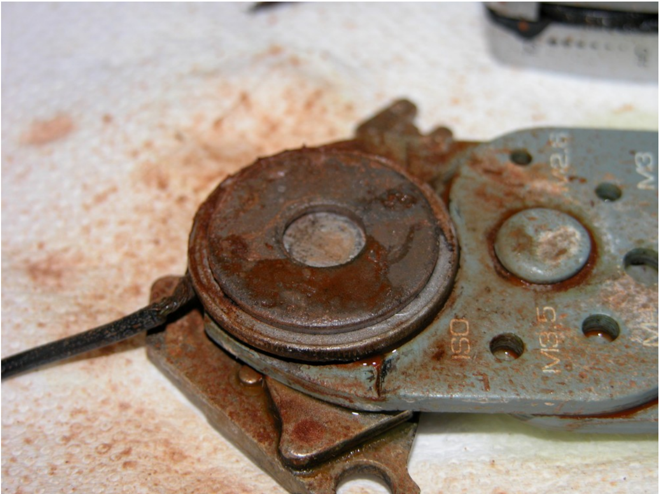
Figure 3.1.4: The exposed electrode surface after attempting to dry up their inner surface (by Joule heating, essentially) does not look substantially different bar for more evident hematite formation.
