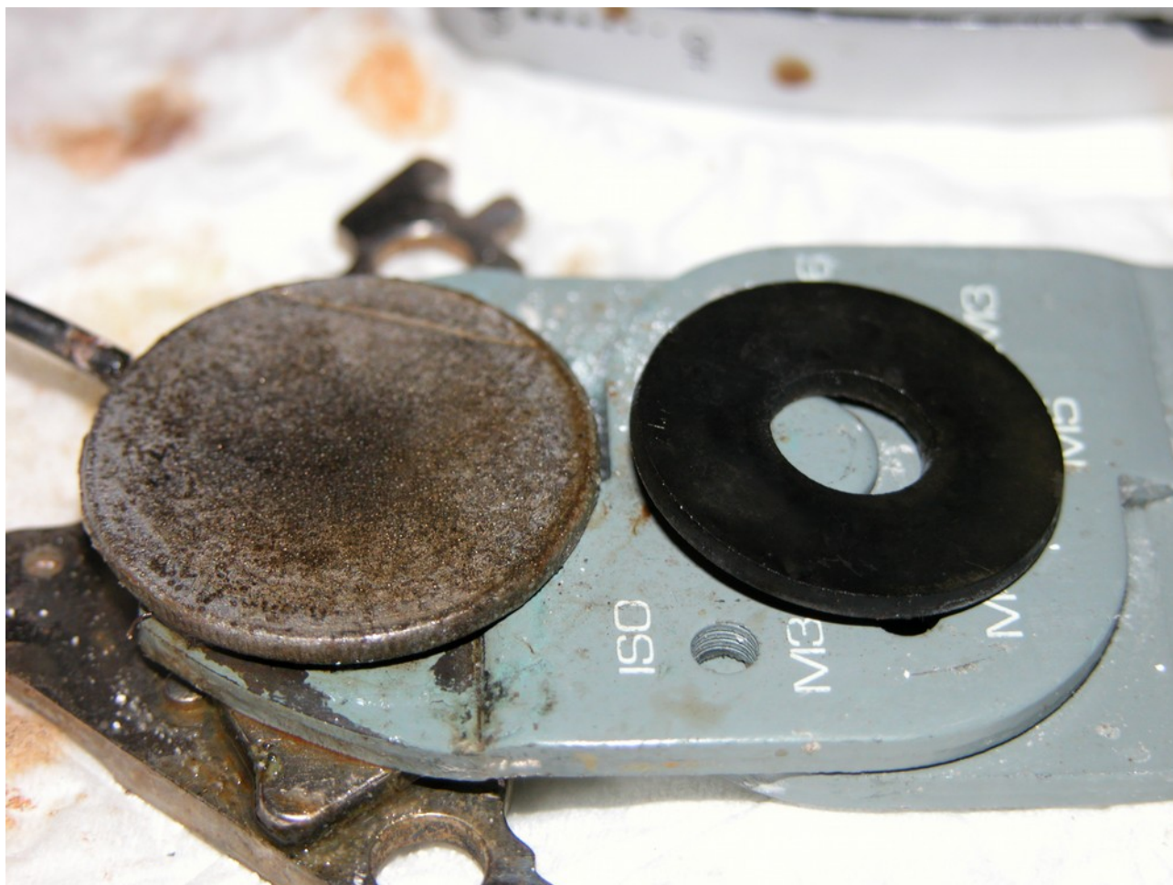
Figure 1.2.4: Conditions of electrodes at the interface after a period of operation. All red iron oxides got removed, cathode became dark black. This arrangement did not prove to be reliable due to the ruined anode surface from previous testing.
