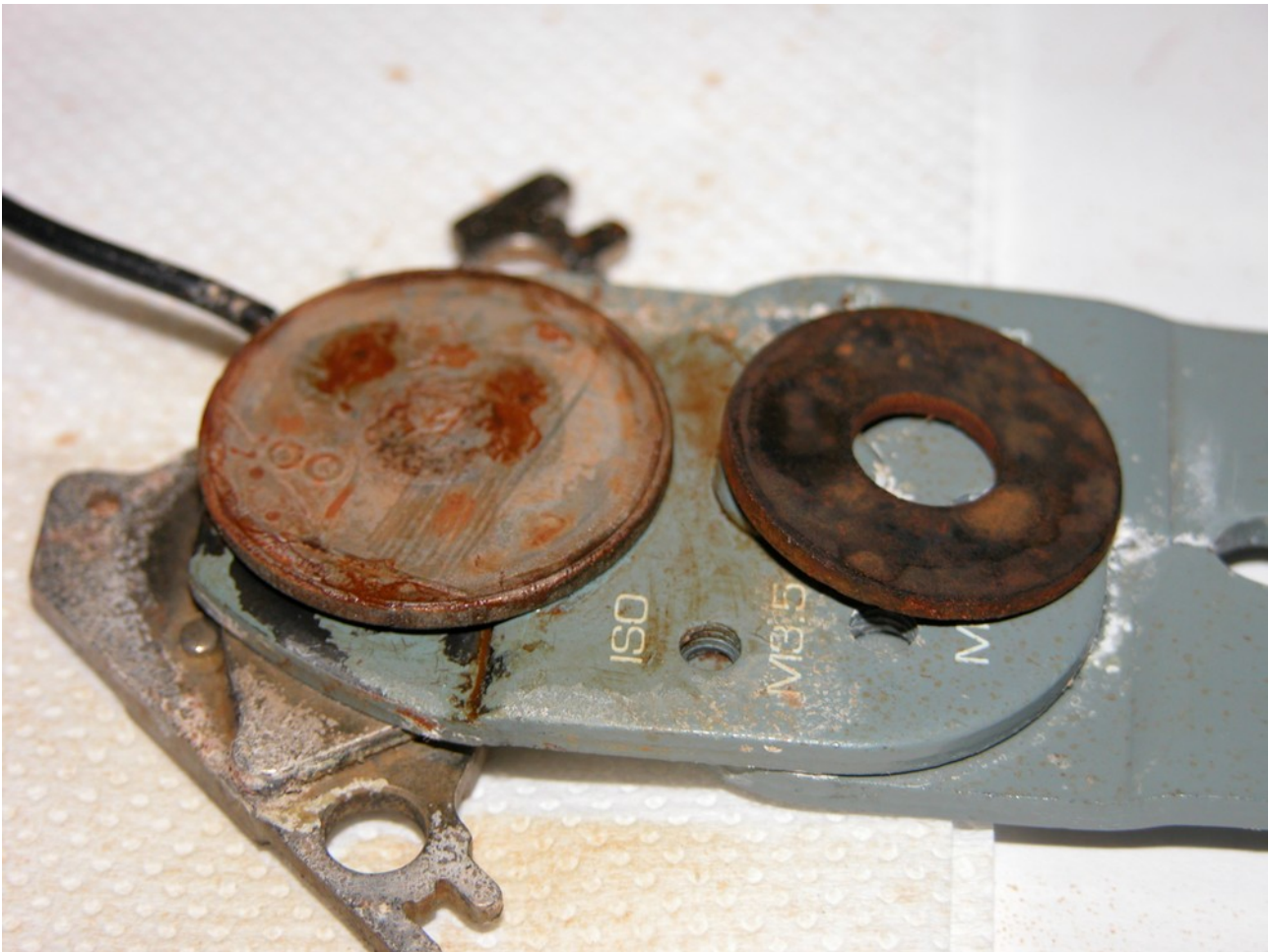
Figure 2.1.2: Electrodes after inspection. At this point there are still relatively large amounts of hematite being produced.
