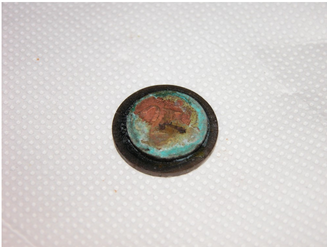
Figure 7.1.1: The coins the day after before separation and after prolonged heating at low temperature with electrolyte solution inbetween.
