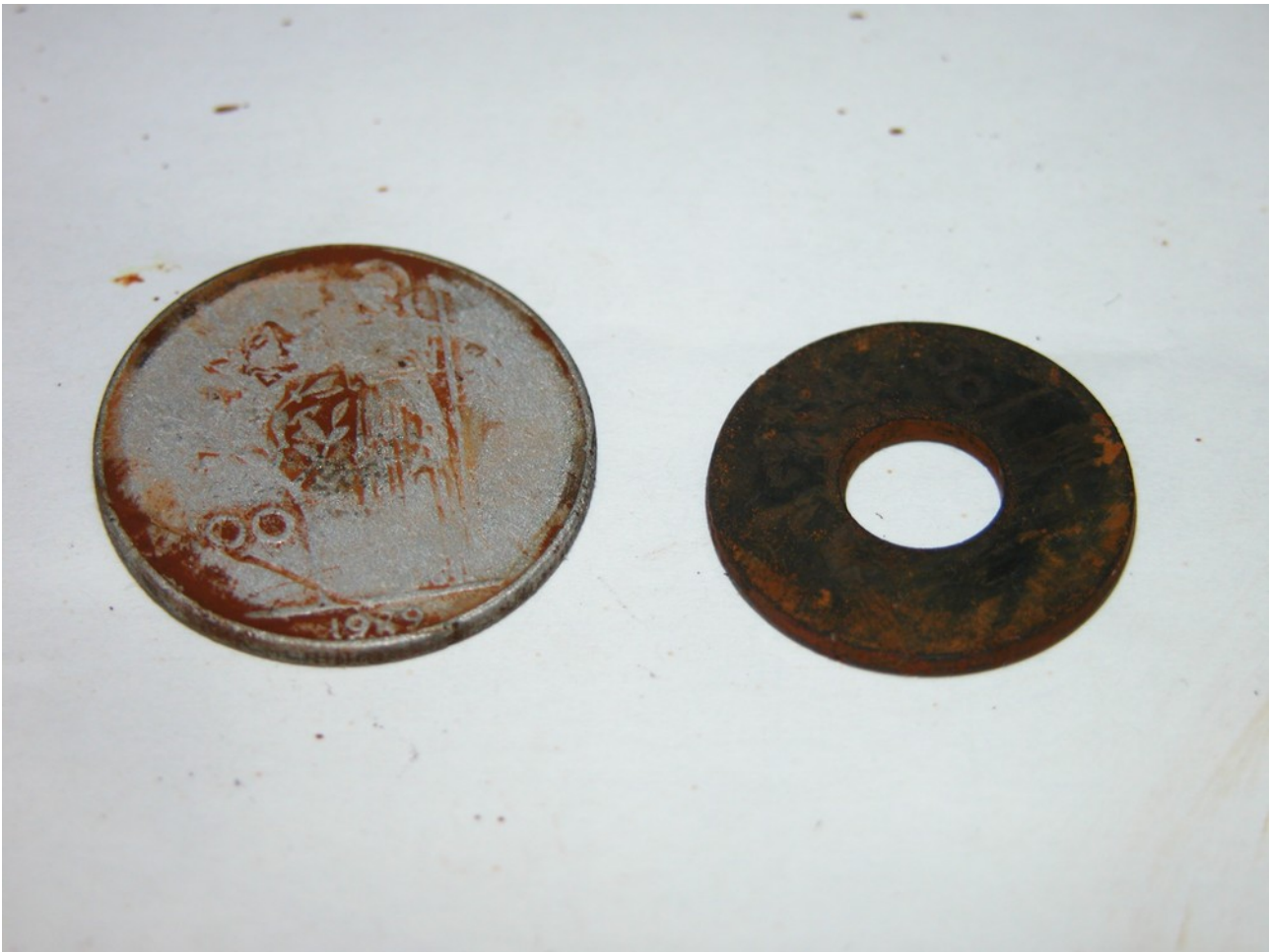
Figure 1.2.7: Electrodes after cleaning in tap water. It's clear that the anode got eroded during the previous process. The cathode got an impression of the anode marking on its surface, and the red iron oxide did not stick.
