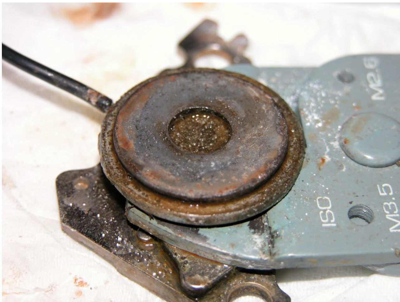
Figure 1.2.3: New electrode arrangement using a 100 Lire coin (SS430) as the anode.
