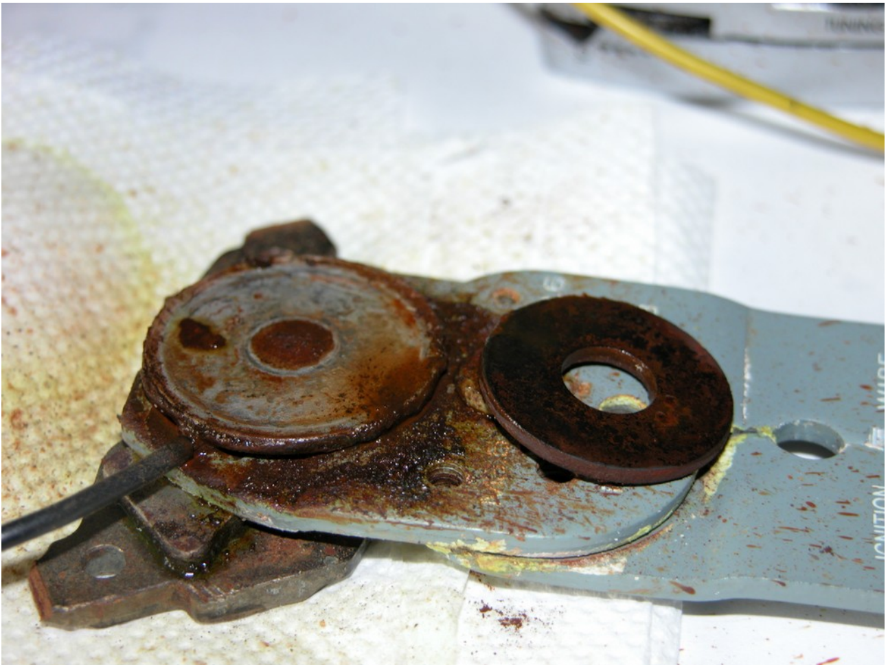
Figure 6.1.4: The electrodes at the interface upon inspection show the typical conditions of the anode getting cleaned (presumably by the evolved gases and steam/cavitation) and the cathode turning dark.
