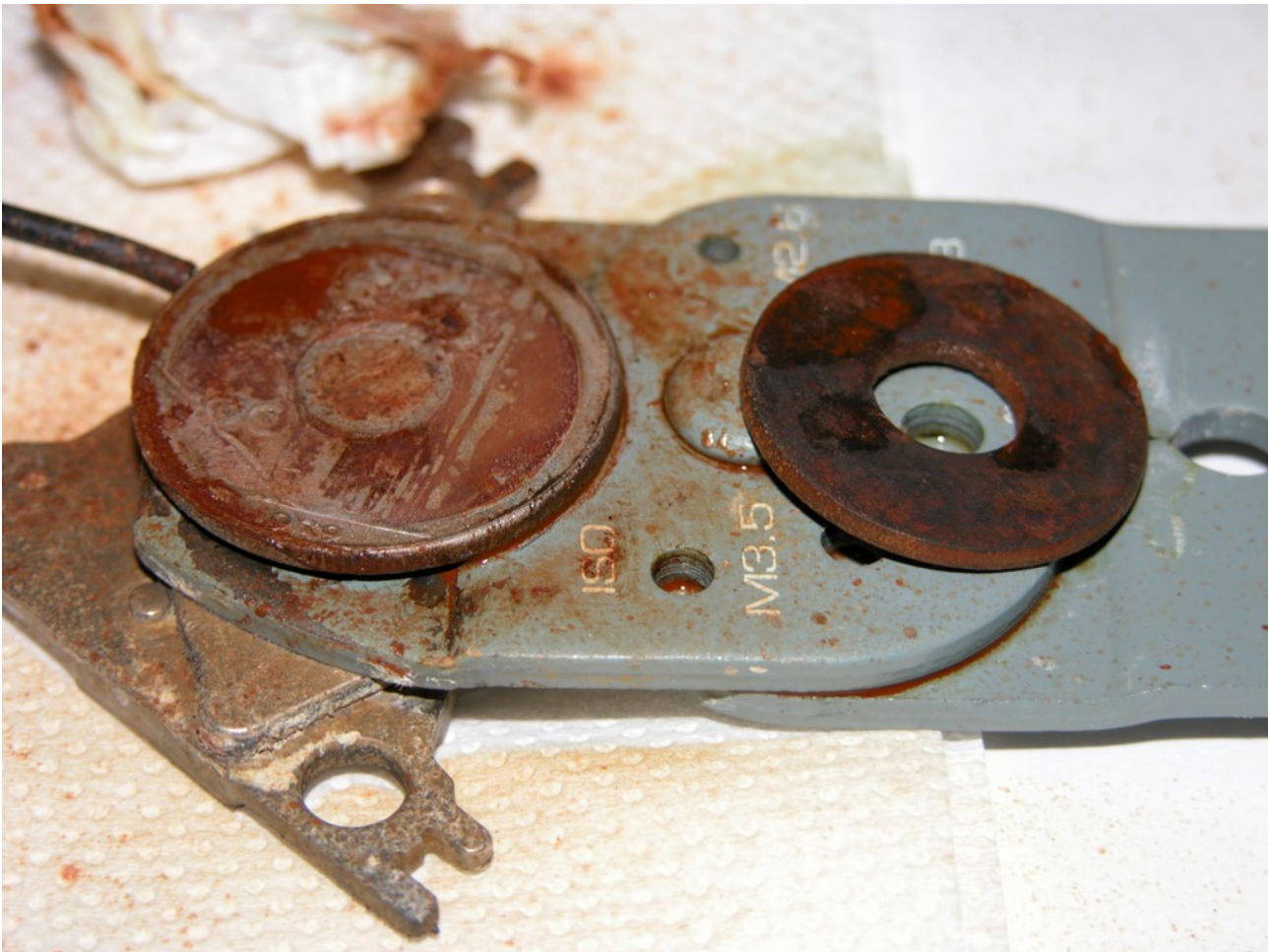
Figure 2.1.4: Red iron oxide (hematite) production decreasing, electrodes kind of getting cleaned after increasing amount of electrolyte in the water solution. It still appears as if upon exposure the cathode turns more reddish.
