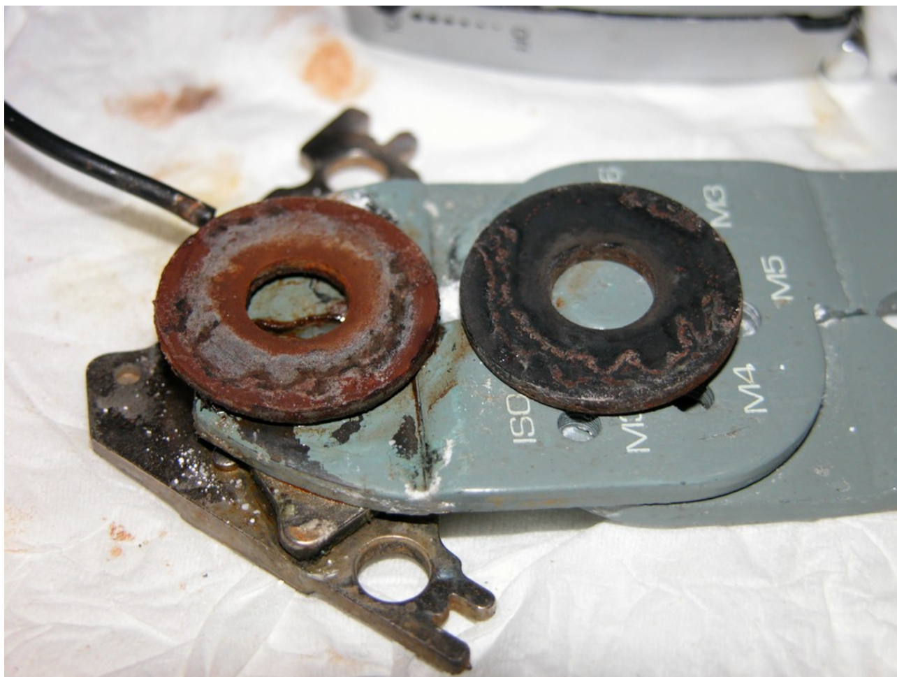
Figure 1.2.1: Electrodes after using a \text{Na}_2\text{CO}_3 electrolyte solution. After a while of operation, the anode got partially cleaned from its surface red iron oxide layer and the cathode became dark black from presumably partially oxidized iron (for the most part).
