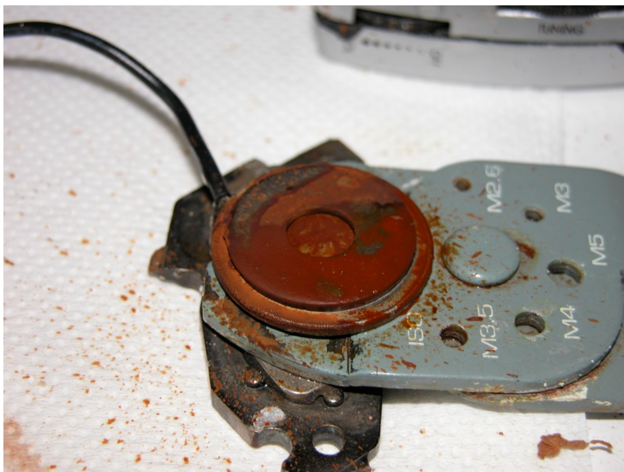
Figure 4.1.3: Hematite formed once the electrode started conducting a current as intended.
