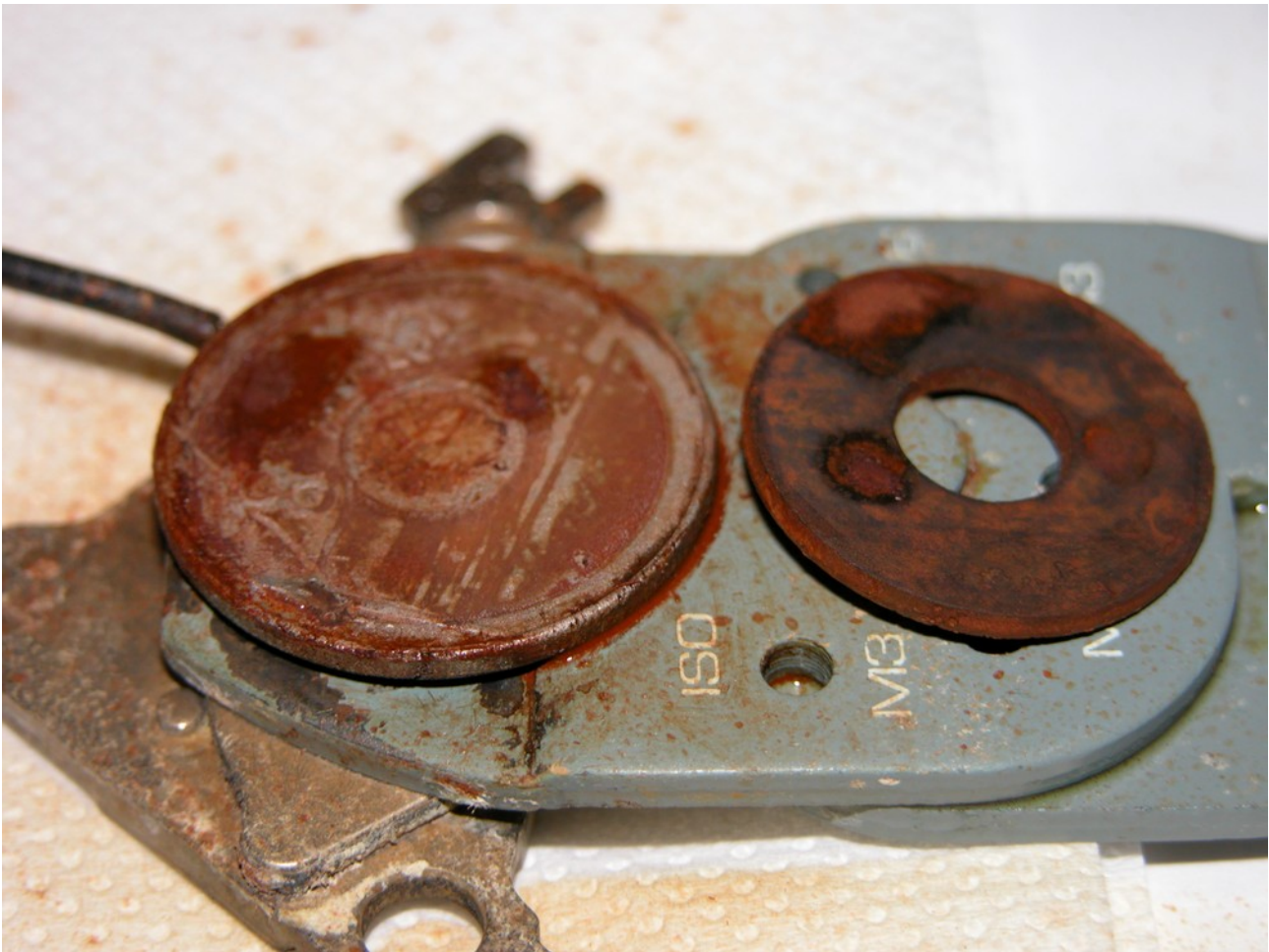
Figure 2.1.3: The cathode quickly turned red after disassembling inspection. Sodium ferrite ( \text{NaFeO}_2 ) production suspected.
