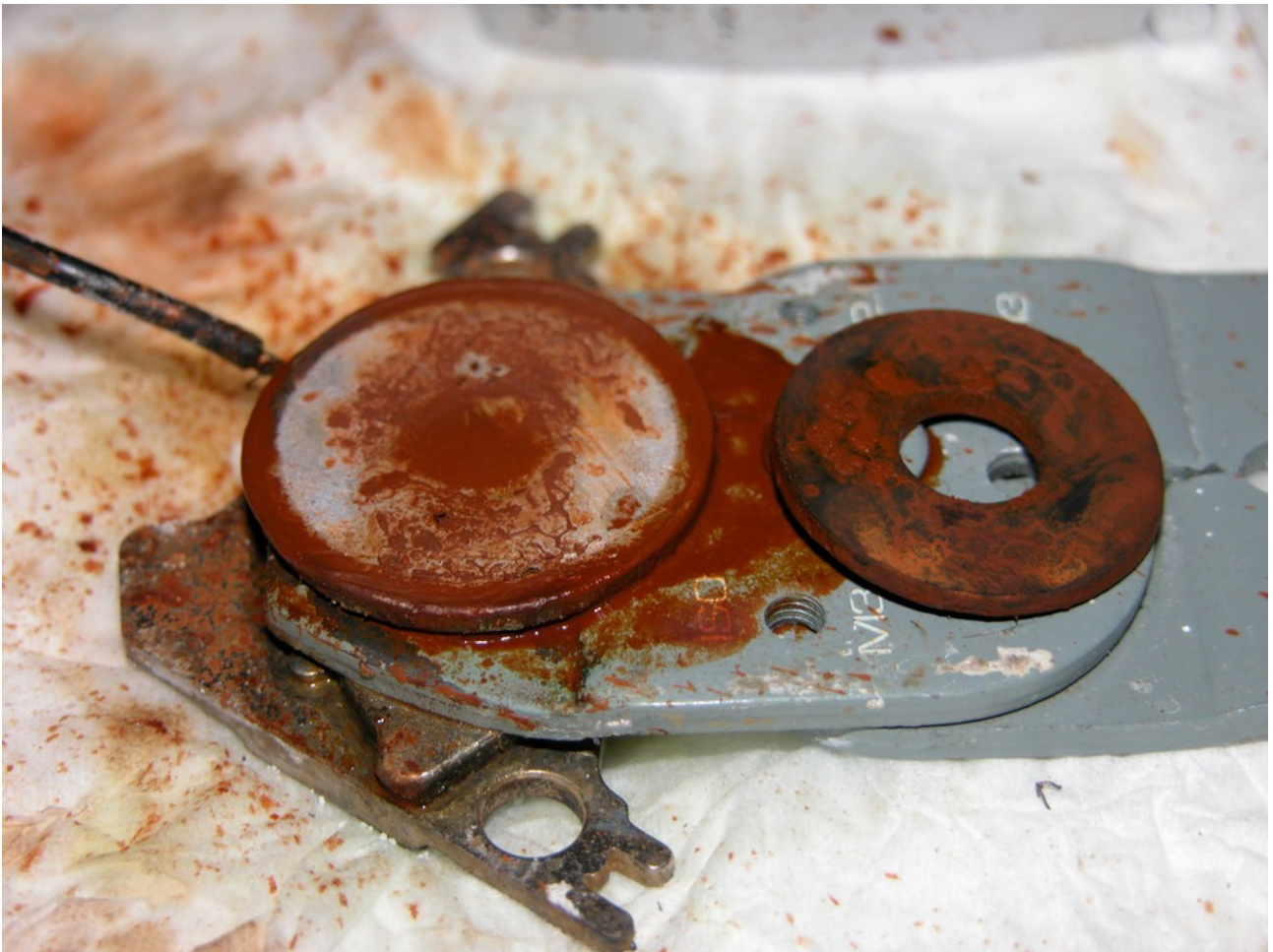
Figure 1.2.6: Both electrodes at the interface. The anode has been cleaned and eroded by the presumably intense cavitating action and gas formation. Red iron oxide is not sticking to the cathode, but the previously formed black oxide (?) layer has remained.
