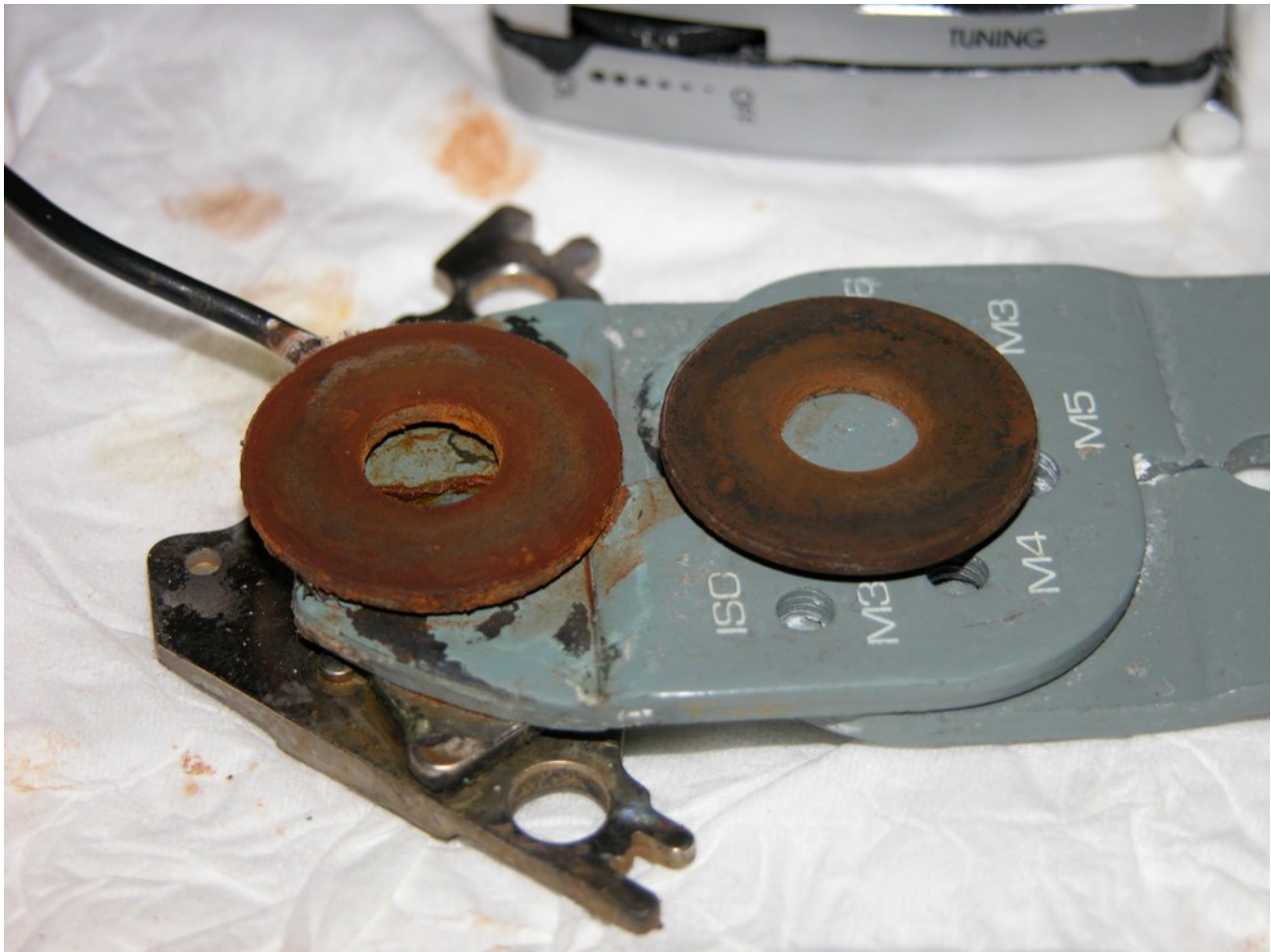
Figure 1.1.2: The electrode interface. When it was first disassembled about 90 minutes earlier, the cathode did not look oxidized like this, but more gray-black looking.
