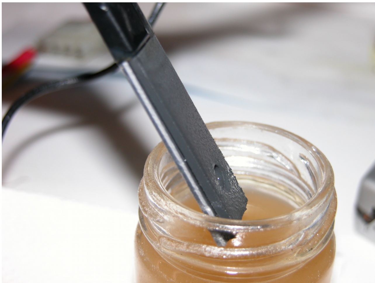
Figure 1.2: The electrode assembly. The gap does not have a fixed width; the assembly is "floating".
