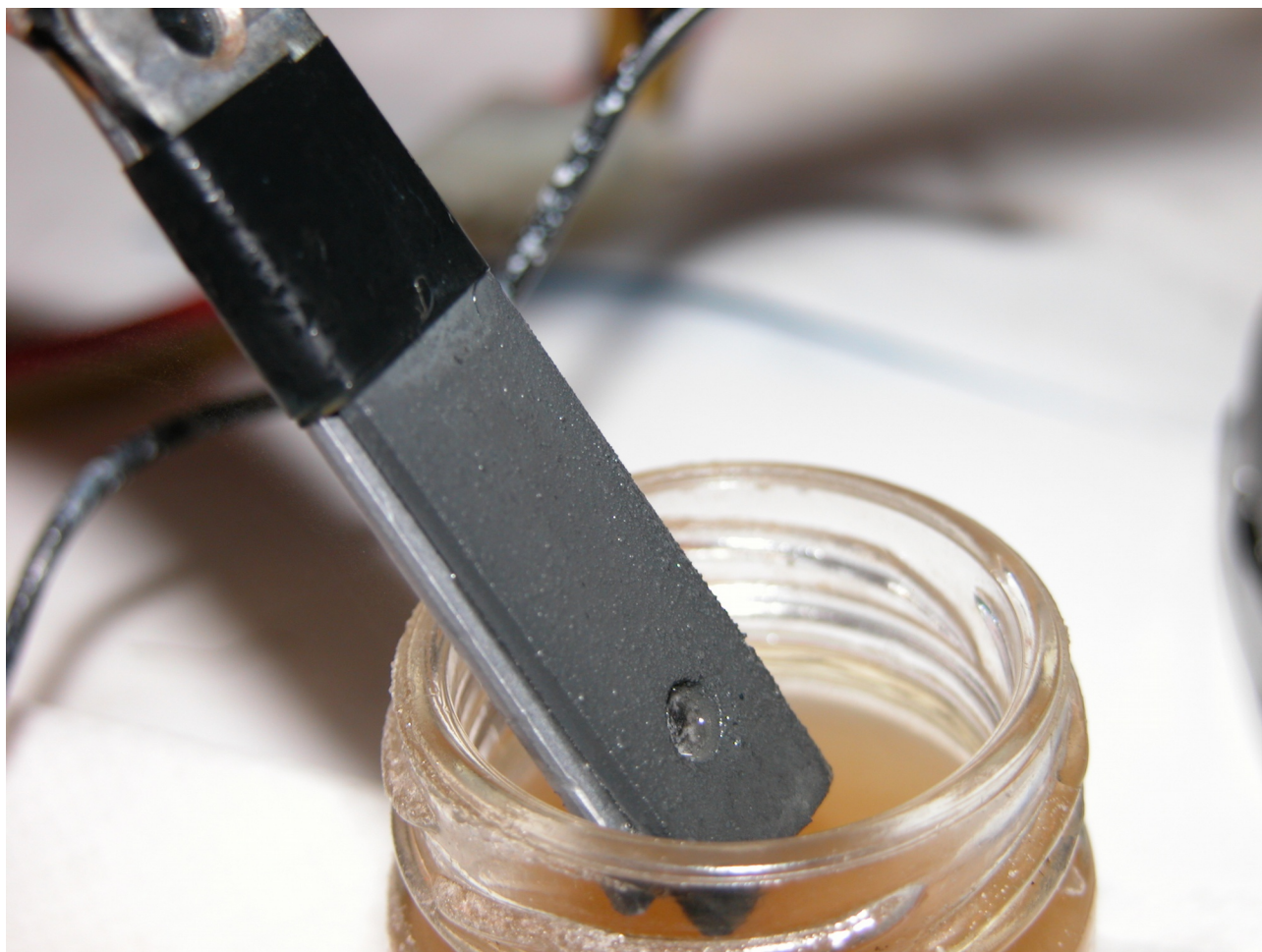
Figure 1.5: The cathode after a longer period of operation.
