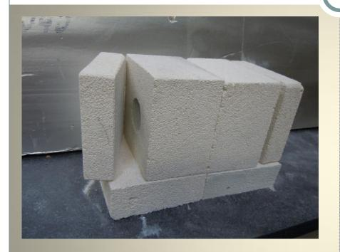
The furnace body is completed by cutting 4x 35mm thick slices from half-bricks, two for the base, one for the removable door and one for the fixed back panel. The final task is to insert the heater coil ensuring that there is enough Kanthal wire exposed to connect to the heating controller. The whole is wrapped in 50mm ceramic wool insulation, and sits on a 25mm pad of wool and another of aluminium foil/foamed urethane.
