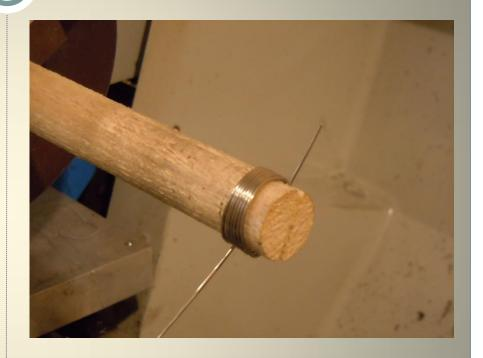
Coils are easy to wind by hand We use an undersize wooden mandrel, in this case 25mm. Coil material cost \$1 approx.
