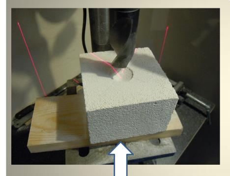
The bricks are cut into two halves and each half bored to accept the quartz tube liner and coil unit. The two bored halves are cemented together using a mix of waterglass zinc oxide and magnesium oxide.
