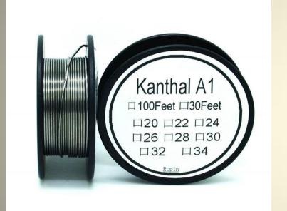
Heater Coils are made from 1mm diameter Kanthal wire 2.4M long. Kanthal is Ni-Cr-Al and has well known resistance characteristics.
