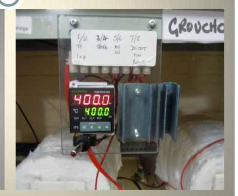
This is the data logger cluster for the 8 reactor bank - every reactor feeds it two thermocouple readings, heater current reading and Geigercounter data. Add in ambient temperature and background Geiger count and we have 34 channels reading once every second.
