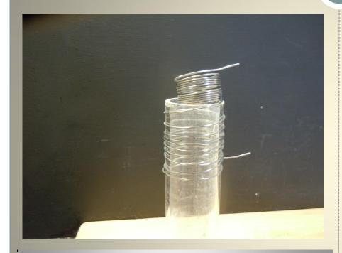
The 25mm. coil is coaxed onto a 40 x150mm quartz tube. The diameter difference ensures the heater coil is In good thermal contact with the quartz along its whole length
