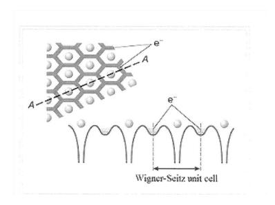
Fig. 2. Schematic electron distribution in Rydberg matter. [5]
