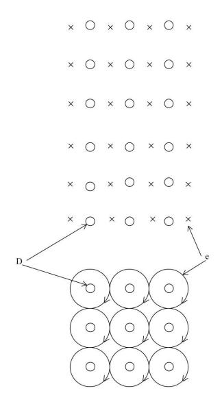
**Fig.4**. Ultradense deuterium- electron vortex tower: D deuterium nuclei, e electron fluid vortices.
