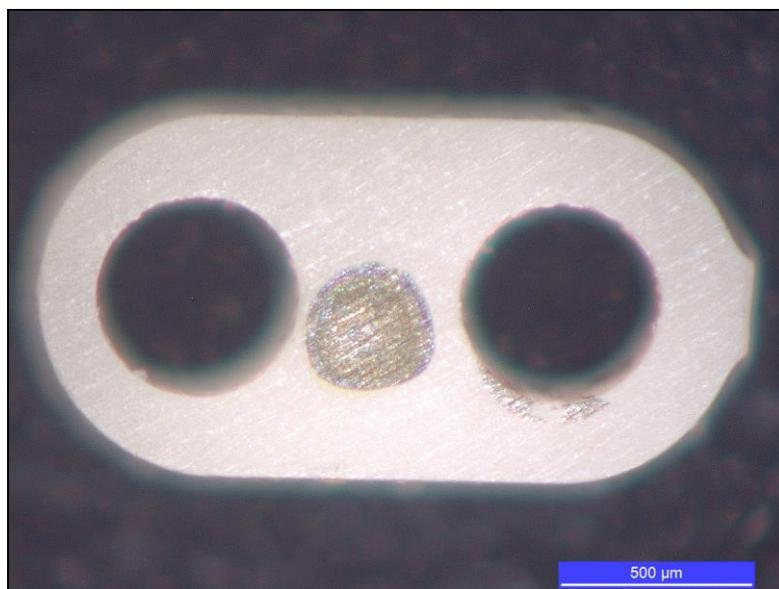
*FIG. 2. Uranium electrodeposited MPFD disk.*
